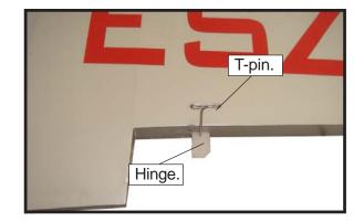
□ 3) Slide the aileron on the wing panel until there is only a slight gap. The hinge is now centered on the wing panel and aileron. Remove the T-pins and snug the aileron against the wing panel. A gap of 1/64" or less should be maintained between the wing panel and aileron.
