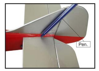
□ 4) Remove the stabilizer. Using a modeling knife, remove the covering from below the lines you drew.
