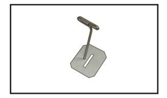
□ 2) Remove each hinge from the wing panel and aileron and place a T-pin in the center of each hinge. Slide each hinge into the aileron until the T-pin is snug against the aileron. This will help ensure an equal amount of hinge is on either side of the hinge line when the aileron is mounted to the wing panel.
