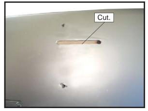
3) Fit the main landing gear legs into the slots in the underside of the wing panels. Position two nylon landing gear straps over each landing gear leg as shown. Mark the location of the screw holes onto the wing and drill holes at your marks using a drill bit. Secure the landing gear legs to the wing panels using the nylon landing gear straps and self-tapping screws as shown.
