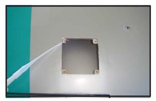
8) A string has been provided in the wing to pull the aileron lead through to the wing root. Remove the string from the wing at the servo location and use the tape to attach it to the servo extension lead. Pull the lead through the wing and remove the string.
